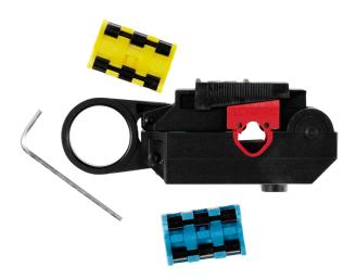
Maxi Corex is a stripping tool for coaxial cable, Ø 7.0-15.0 mm/0.28-0.55", 3 blade, stripping length 9.5 + 3.2 mm/0.374 + 0.126".
